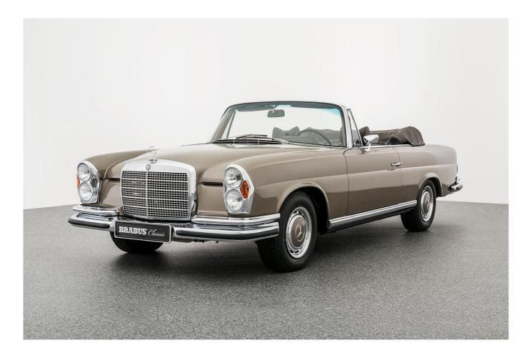
Power 147 kW / 200 PS | 0-100 km/h 9,4 s | Vmax 205 km/h / 127 mph Fuel Economy\* city - l/100km | highway - l/100km | combined - l/100km | CO $_2$  - g/km
